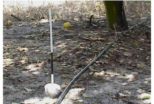
Most flatwoods citrus soils have a restrictive layer that can perch the water table and significantly affect tree water relations. To optimize production and tree health, the level of this water table should be monitored and maintained within an optimal zone. Simple and practical observation wells can normally produce adequate information.
