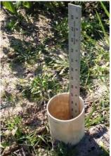
Most flatwoods citrus soils have a restrictive layer that can perch the water table and significantly affect tree water relations. To optimize production and tree health, the level of this water table should be monitored and maintained within an optimal zone. Simple and practical observation wells can normally produce adequate information.
