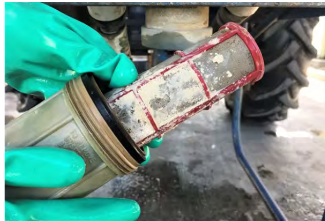
clogged sprayer filter
