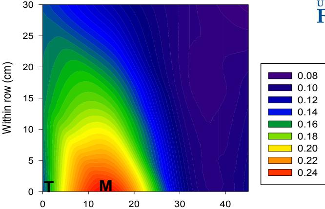
Cross-row (cm) Lateral root density (cm cm<sup>-3</sup>) distribution using ACPS microsprinkler
