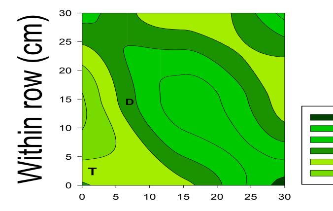
Higher NPK conc. in irrigated vs. non-irrigated zones of drip fertigation. D=area below dripper, T=tree
